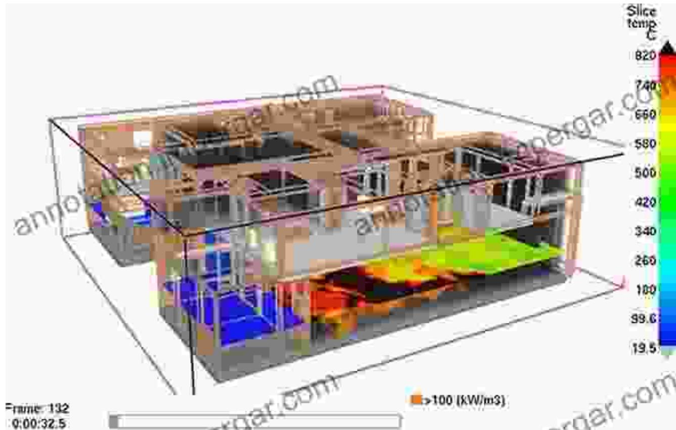
CFD Simulations: Harnessing computational power to visualize and analyze fire and smoke behavior.
